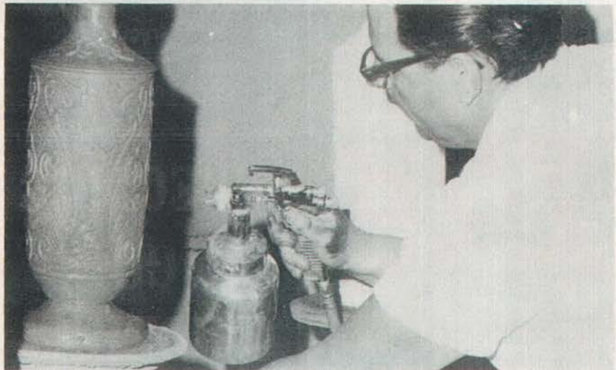
Ernest Silcox of Route 7, Carthage, puts the finishing touch to a Neda lamp after it comes out of the furnace which hardens the hydrocal base for better strength and protection.
