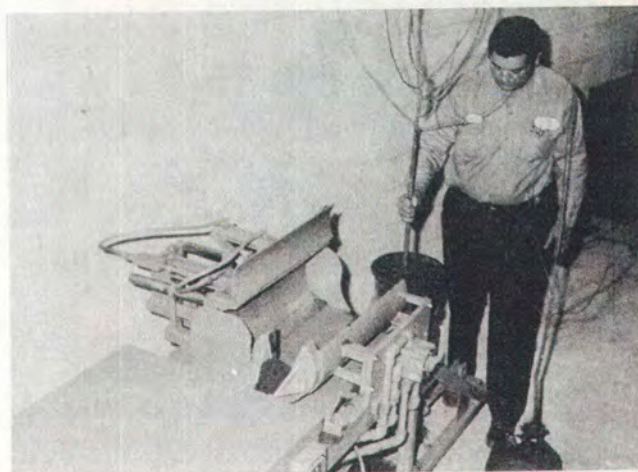
Avery Lawson with ball and potting machine which will run about 150 units per hour.
