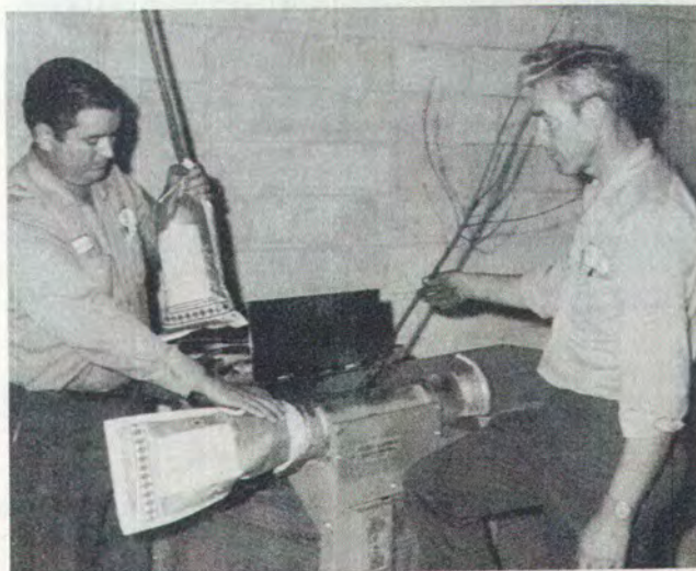
Left to right: Avery Lawson and Elbert Bouldin demonstrating a nursery packaging machine. The machine speeds packaging of plants 10 times faster than the old method.
