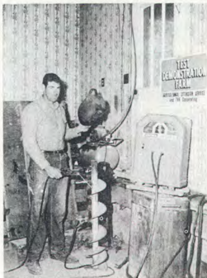
R. E. Scarbrough, Jr., in his farm shop preparing to make an electric weld on the auger of his handmade, tractor power, take off post hole digger. Electric equipment in this corner of the shop includes an air compressor, battery charger and electric welder.
