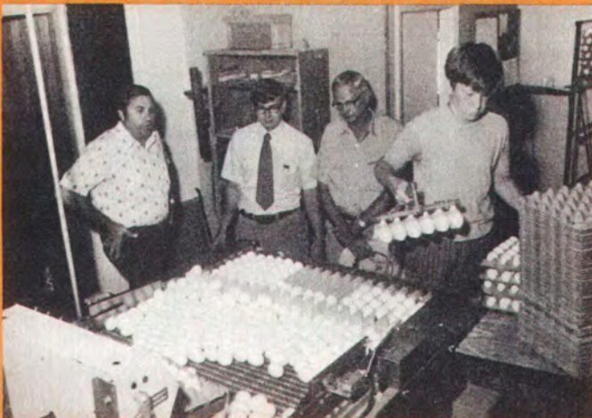
From left to right, John Ashby, General Manager of Hudson Brothers, Inc.; David Joiner, Consumer Services Representative of Cumberland Electric Membership Corporation; and Bill Hudson, partner in Hudson Brothers, watch employee lift eggs by vacuum at central collection station for placement on flats. Eggs will go immediately to cooling room, then to processing plant soon thereafter. Cumberland Electric provides the power for this sizeable electric load, including laying house and processing plant.
